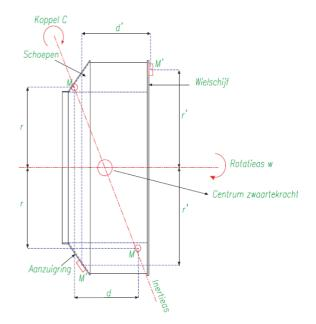
The grade, notion frequently used, is a quality of impeller balancing which allows calculating the residual acceptable unbalancing, according to nominal speed when we work on the machine to be balanced. The most used ones are G 6.3 (small size machines) and G2.5 (larger machines).
