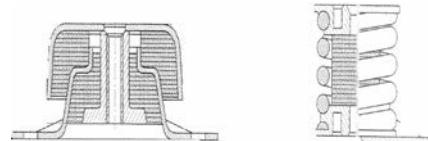
*The rubber isolators are made for example with natural rubber wedged between metal frames of variable stiffness depending on the model. Or in a form of springs, sometimes very flexible; particularly suitable for fans working at very low speed.*
