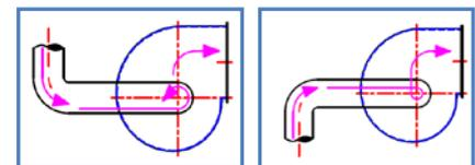
Ex 2 : A damper installed too close to inlet's fan. The damper will create a distortion of the air flow, generating an irregular load on the impeller. A damper should be installed at least at 5D (D= Ø of the duct) of the inlet flange, in order to allow the air being redistributed correctly before to enter in the fan.
