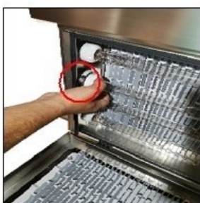
5. Remove the UV lamp from the socket and change it for the specified type according to the specification.
