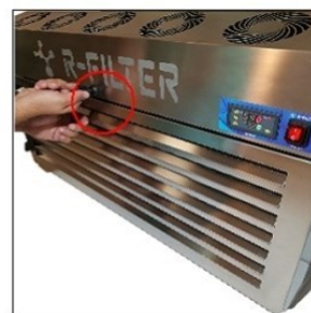
6. Close the service door, turn the key to locked direction.
