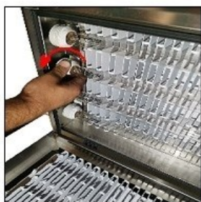
4. Unscrew – anticlockwise- the retaining rings of the selected UV lamp separately.
