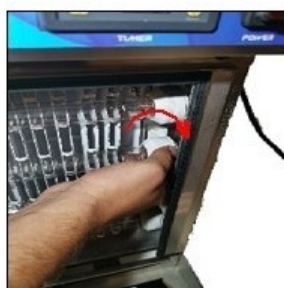
6. Close – clockwise- the retaining rings carefully to ensure their proper protection. Clean the lamps if needed.
