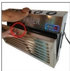
7. At closing the service door, check the exact fit.
