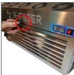
8. Close the service door, turn the key to locked direction
