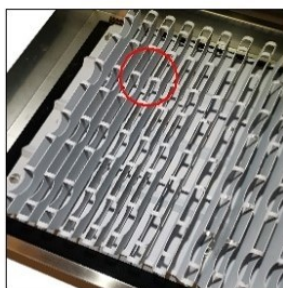
5. Check the internal surfaces for cleanliness.
